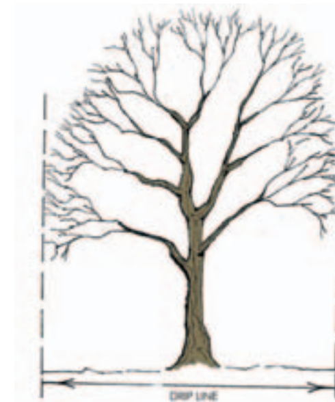
Trees to remain within the Limited Disturbance Zone shall be protected from any damage and should be delineated with orange construction fencing around the drip line of the trees.
