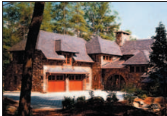
Sensitive thought must be given when locating the garage. The roof massing and detailing help downplay the potentially overwhelming presence of the garage. The front door remains the focus as one approaches the house.
