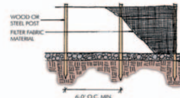
All erosion and sediment control measures such as silt fences shall comply with all local and state regulations.
